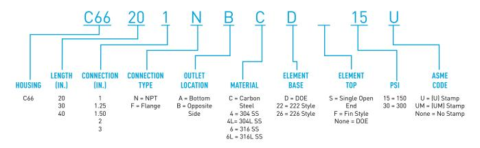
Note: If DOE, it is only required once in the part number and will specify both top and base. Cartridges are not included but must be specified as to the type using when ordering the housing. Carbon steel not recommended for water use as the epoxy coating is not designed as a corrosion inhibitor.
