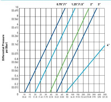
Flow Rate – gpm (Lpm)
